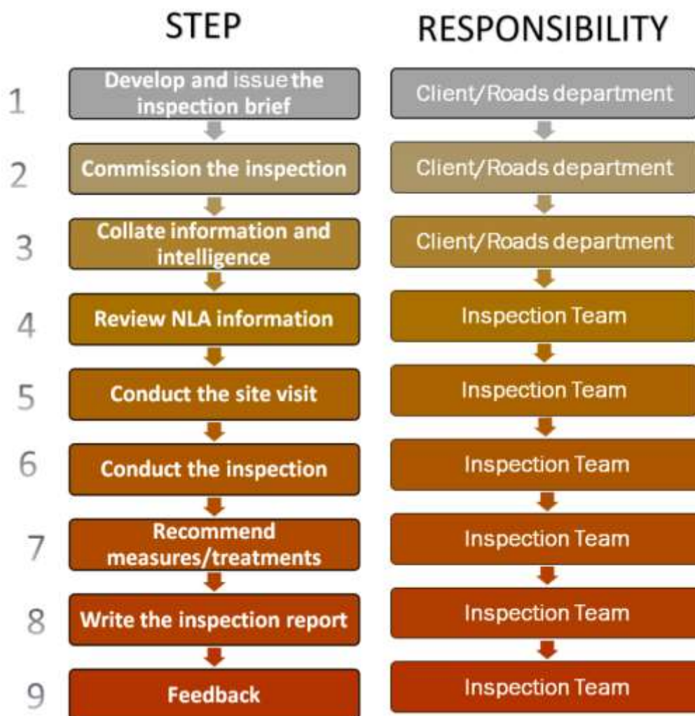
Figure 4-2: Inspection process flow chart
