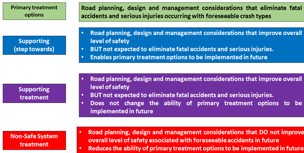
Figure 4-3: Treatment hierarchy (NZ Transport Agency, 2013; (Austroads, Guide to Road Safety Part 6A: Implementing Road Safety Audits 2019)
